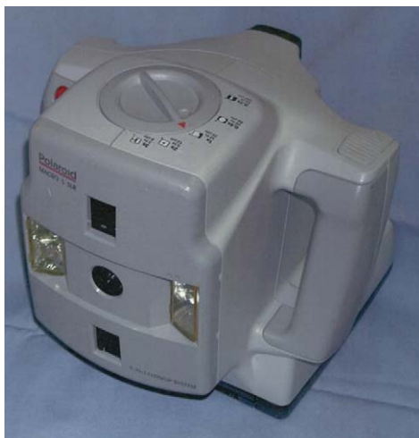
Fig 2. Polaroid Macro 5 SLR camera. Note the dial for choosing the magnification on top of the unit, and the two integrated front flashes.
